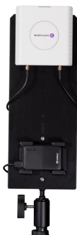
Figure 33: connect the two TNC/SMA cables on the IP-xBS SMA antenna connectors then connect to the IP-xBS to its battery, mount the IP-xBS on its support.
