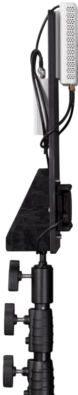
Figure 34: fully assembled fixing plate connected to the tripod
