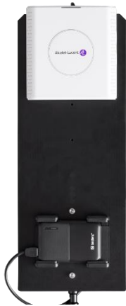
Figure 28: mount IP-xBS on its support
