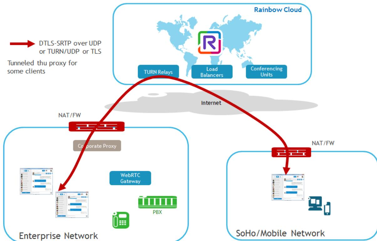
Note: to simplify figures, only one TURN server is illustrated. For a P2P communication, depending on geography and network performance, up to two TURN servers could be used to establish a communication (a different one for each client).
