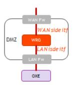
Should the WebRTC Gateway be deployed in a DMZ, make sure the following requirements are addressed:
