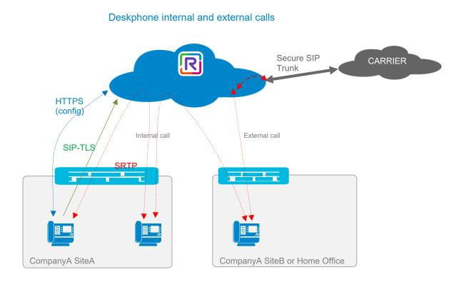
The configuration file contains the SIP parameters that then allow SIP devices to register to the platform through the nearest SIP entry point, and consequently establish the signaling link based on SIP-TLS. The SIP-TLS link is always to the initiative of the device and maintained permanently with the Rainbow back-end thanks to keepalive traffic sent over the SIP-TLS connection.
